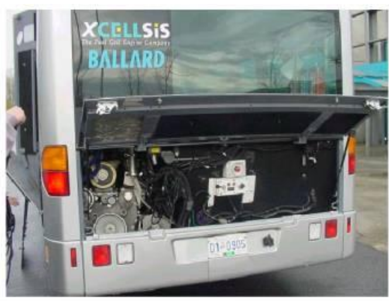
Figure 5. The fuel cell system is housed at the rear of the bus. The compressed gaseous hydrogen is stored in tanks on the roof of the bus.
